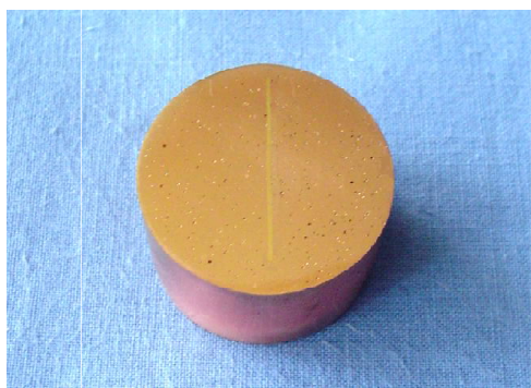
Slika 2. Uzorak obložen zlatom Figure 2. A gold-plated sample
