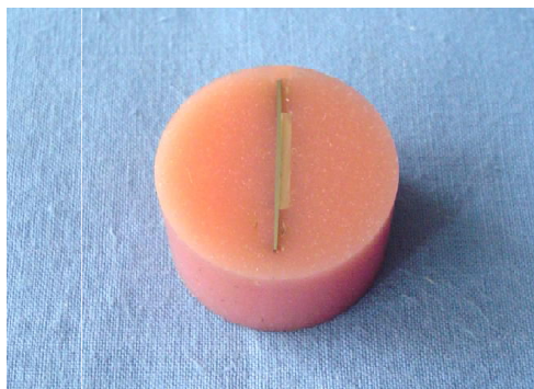
Slika 1. Metalografski ispoliran metal-keramički uzorak Figure 1. A metallographically polished metal-ceramic sample
